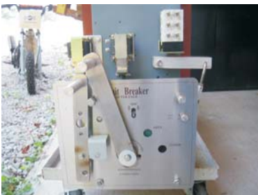
New faceplate, auxiliary, and solenoids on Ensign/LinePower style circuit break switch
