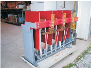
Reconditioned Ensign/LinePower style circuit break switch
